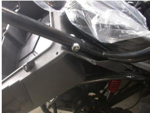
2.13 Joint the front and rear roll cage: joint the roll cages and connect them with M8x30 bolt and M8 nut. The recommended torque is 22-29NM
